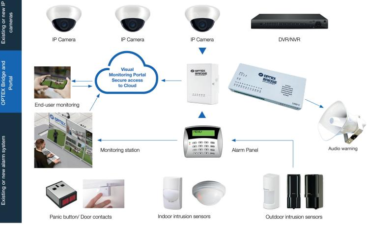
(Compatible with any OPTEX or third party indoor and outdoor detection sensors, door sensor and panic alarm)
