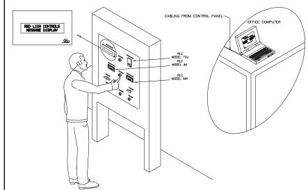
The TCU, IMH, and IMI are set up to activate their alarm outputs in the event of an error condition. Each output is tied to a separate data pin on the parallel port of the ADI. The ADI will automatically request a specific Message from the parallel port when a level change occurs.
